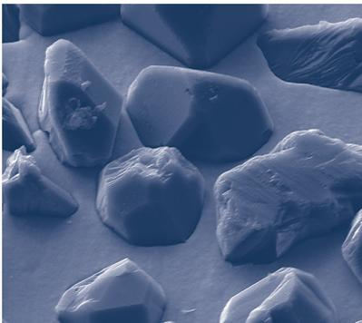
Abrasive coatings, which are applied to the base body with a thickness of 0.65 – 1.5 mm occupy an exceptional position in the world of electroplated coatings. The bonding and cutting properties of this abrasive coating are comparable with those of a sintered bronze bond.
