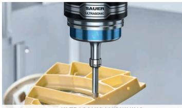
ULTRASONIC MACHINING ULTRASONIC 2<sup>nd</sup> Generation Most efficient way of machining hard and brittle material.
