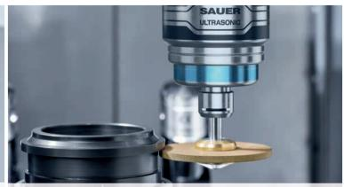
CYLINDRICAL GRINDING Mechanical seal (SiC) ID / OD, pocket, and threading processed in one setup.
